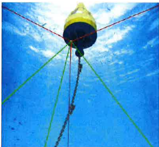
A standard current profiler cannot measure the complete profile from the bottom to the surface. Instead, it loses data close to the instrument and close to the far boundary. The Aquadopp Z-Cell extends the profiling range by introducing a «Cell Zero». The data is generated by an extra set of horizontal transducers. The transducers operate at a different frequency (2 MHz) and provide the 2D current velocity at the level of the instrument. This is to the benefit of anyone who is interested in the detailed current velocity in the boundary layer.
